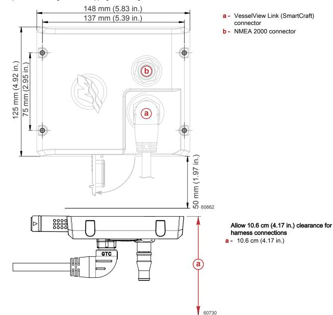
3. Use a #29 drill bit (0.136 in.) to drill the four pilot holes to mount the VesselView Link module.
